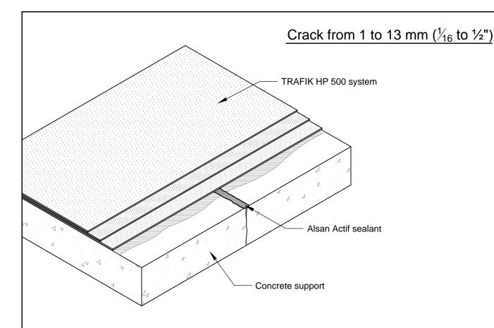
Note: Rout out minimum 6 mm (1/4") wide and fill with polyurethane sealant
